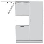
"X" approx. 48,0mm (old 35,0mm) (x = distance from top edge of wall unit to hole (centre) in mounting rail).
